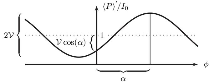
Fig. 1: Interference pattern of the probe expectation value. For a suitable choice of probe parameters, destructive interference at the origin  $\phi = 0$  witnesses entanglement between the two target qubits.
